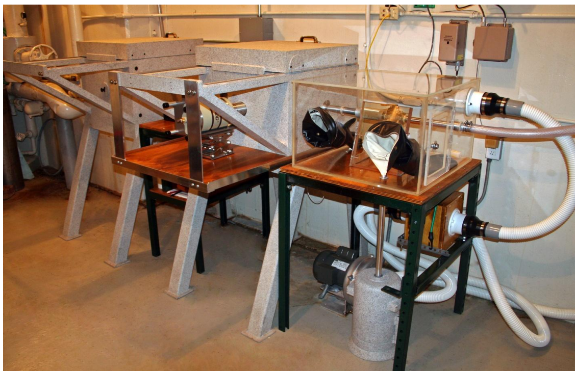
Fig. 9. Hot Cell System with HPGe Detector
