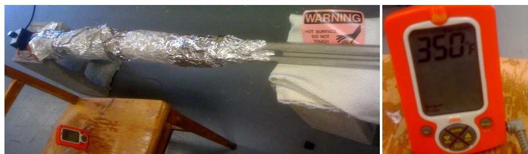
Fig. 4. Heat Treatment of In-Core Assembly
